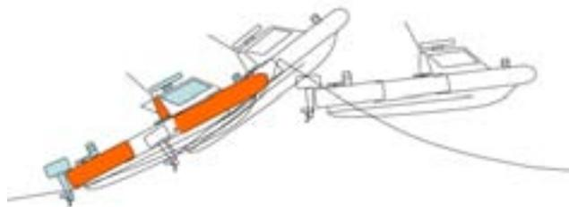
The most direct course to the destination may not be the best course to follow (diagram opposite). Angling the CRV to the line of the waves has the effect of lengthening the distance between crests. This can produce a much more comfortable ride.
