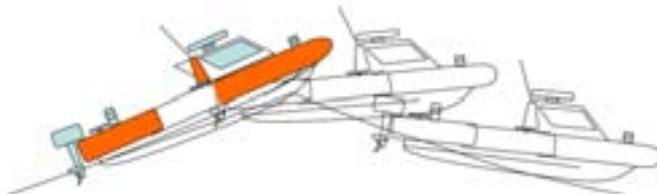
In more adverse conditions, it may be impossible for the helmsman to prevent jumping when travelling at speed, but a good angle of re-entry should be aimed for. Ideally, this angle should not exceed approx 30° off the horizontal.
