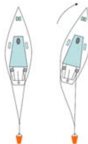
The problem can arise however that the steering is not simply broken (in which case the rudder / drive systems can often be secured in a central / midships position), but that the steering is actually jammed at an angle. This may be due to damage incurred when hitting and object, or if a rope / fishing gear has become entangled in the rudder.
