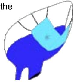
Positioning the fothering / collision mat can be tricky, and any lines attached to the mat usually need to be weighted so they will drop under the vessels hull. A triangular shaped mat like the one shown opposite is often far easier to position and secure
