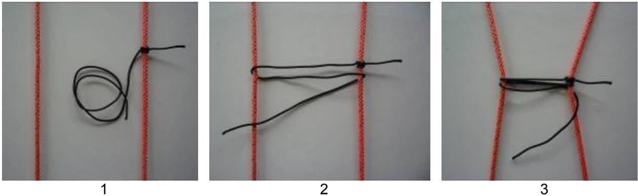
As the gap between the main lines is reduced their tension / loading will increase. Each 'frap' is like a small block and tackle being used – the cumulative effect is that by frapping with even a very small diameter line, the loading on the main line(s) can be increased many times more than by just hauling tight by hand or using a Waggoner's hitch.
