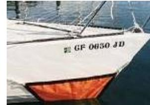
Any movement through the water either by towing the distressed vessel, or them making way under their own power will probably displace the fothering / collision mat – but again it may buy you valuable time in which to come up with a more permanent fix.
