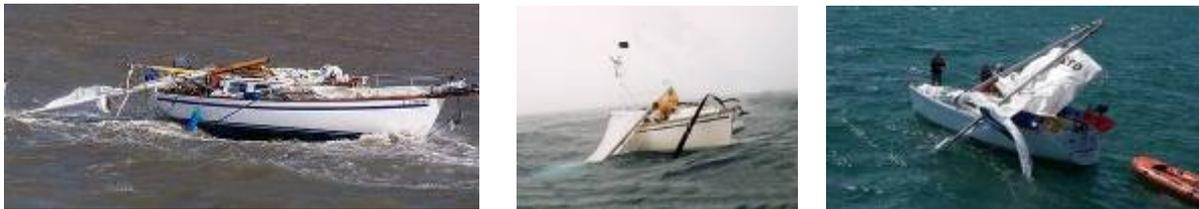
Any assistance given to a dismasted vessel must be approached with caution. There may be ropes trailing from the damaged rig in the water. The damaged rig can become a tangle of moving wire & rope under tension, and any attempts to cut away or secure the broken rig must be made methodically and carefully.
