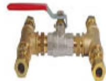
In the event of a seizure or breakage in another part of the system this by pass valve may need to be opened to allow the rudder / drive systems to move freely. This would be preferable to a steering system effectively jammed at an angle. With the rudder / drive system working freely an alternative method of controlling steering might be employed, such as emergency tiller (if the vessels has one) or the rudder(s) secured amidships by lashing / clamping the rudders stock, quadrant or rack.
