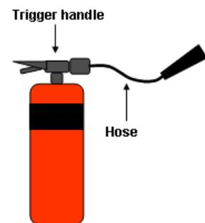
The cones usually found on the end of a CO2 extinguisher's hose have occasionally been known to blow off the end of the hose when the extinguisher is activated.
