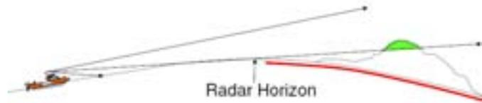
To work out the Radar horizon for particular Radar, take the square root of the scanner height in metres, and multiply by 2.2 to obtain the Radar horizon in nautical miles.
