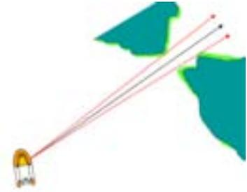
In the diagram opposite, the distressed vessel is anchored less than 200m from the shore, and because of the beam width its radar image merges into the image of the nearby headland. At a distance of a mile the CRV may not be able to see the vessel.
