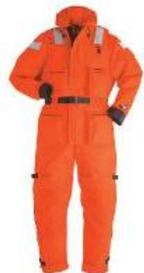
The added floatation in the suit also means that it takes a far larger lifejacket to turn the wearer face up. The typical buoyancy of most 'offshore' inflatable lifejackets is 150 Newton's (15kg of buoyancy). Many floatation suits need lifejackets of 250 – 275 Newton's to turn a person face up in the water.
