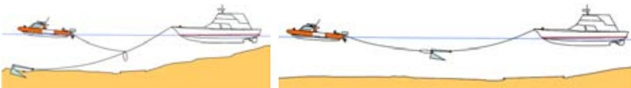
The tripping line should be allowed to sink to the sea bed and the pull from the CRV should be as horizontal as possible. If the tripping line from the CRV is pulled too hard, or the anchor rode from the anchored vessel has very little weight / pressure on it then there is the chance the tripping line will snag on the rode before it has reached the anchor (diagram right).
