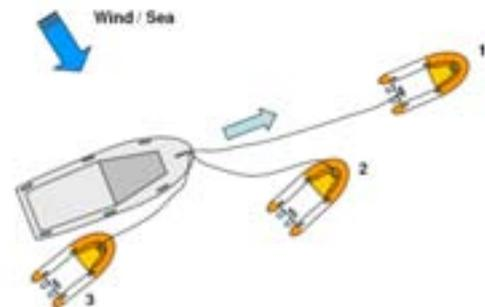
While manoeuvring the CRV gather in any slack or pay out on the tow line accordingly to prevent the tow line catching on any obstructions, and to keep it clear of the CRV props / jet units (jets are particularly prone to 'swallowing' lines in the water). If the attempt to go alongside has to be abandoned for any reason, with the towline still attached control of the tow can be regained and the manoeuvre attempted again.
