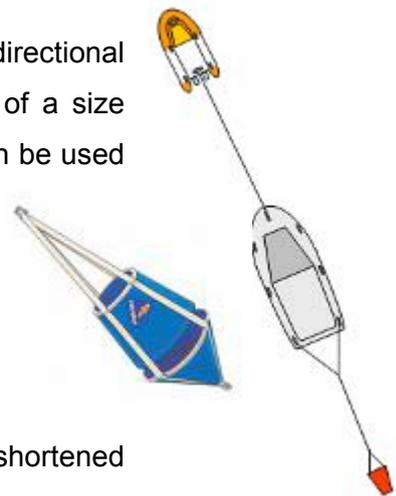
Drogues can be of particular use when a towline has been shortened up in preparation to enter harbour, when running a bar, or when towing in a following sea.
