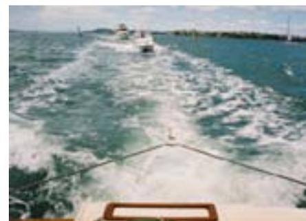
With the first method the main towline is a set length and any adjustments to the towline length are made with the bridle line. The disadvantage is that to lengthen the towline by 5m you may end up paying out almost 10m of bridle line. The advantage is that the strain of the tow will be equally divided between the two quarter cleats.
