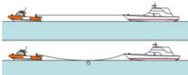
This weight or catenary device may be a permanent feature, such as a length(s) of chain in the towline, or a weight that can be added to the towline as required.
