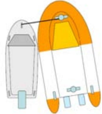
With vessels that are larger than the CRV the position of the CRV relative to the other vessels becomes more important. With larger vessels, as the CRV comes alongside the most important line to secure first is often the bow (forward) spring, followed by the stern line then bow line.
