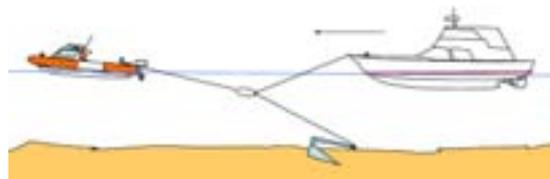
If the tripping line does snag on the anchor rode, it will tend to pull the anchored vessel towards the tripping line. This will eventually exert a pull on the anchor, but it risks damage to the anchored vessels bow (due to contact with the tripping line chain / anchor rode), and tripping the anchor in this way is not as effective as pulling directly with the tripping line.
