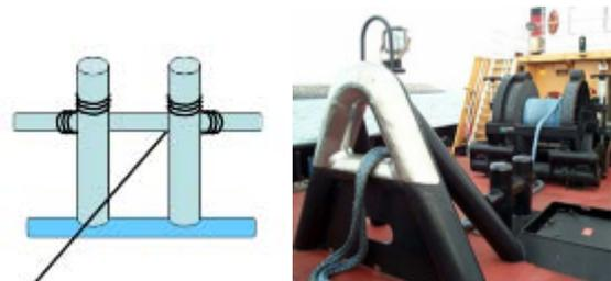
***All CRV crew should be aware of the potential hazard of the towline parting and its subsequent recoil. Great care must be taken to ensure the towline is stowed correctly and is free to run at all times.***
