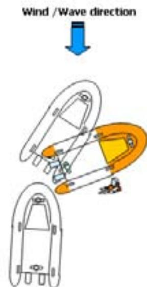
If the PIW is conscious and uninjured, contact may be made with a messenger line. The PIW slowly pulled toward the CRV, with the engine(s) put in neutral, and the PIW assisted aboard.
