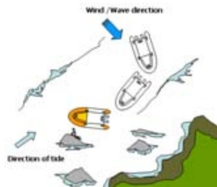
Going alongside a stranded vessel can be fraught with all manner of dangers. The Skipper must consider both the best method of approach to the vessel aground, and the best position alongside for transfer of persons - a point of low freeboard, clear of obstructions and with no overhanging hazards. Debris floating close to the stranded vessel may damage the CRV or foul its drive units. The vessel might have deployed an anchor before grounding and its anchor rode may be just under the surface.
