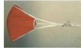
A sea anchor is designed to stop a vessel completely, or at least reduce its drift to an absolute minimum, and therefore is larger than the drogue and normally deployed off the bow.
