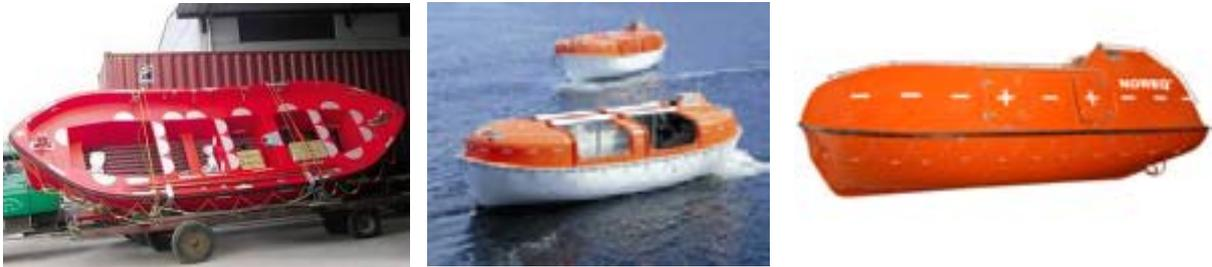
The transfer of persons from lifeboats, especially totally enclosed lifeboats has always presented particular problems. Lifeboats in general by the nature of their construction and design are usually very buoyant and lively at sea. The motion a lifeboat may have, even in moderate conditions can make transfer of personnel extremely difficult.
