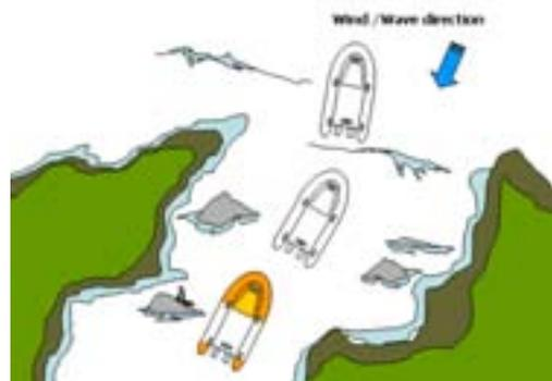
In moderate seas it will usually be possible to drive the CRV astern, giving short bursts ahead to correct any steering problems. In adverse conditions it may be better to allow the CRV to be washed back into the inlet, using both astern and ahead power to control steering.
