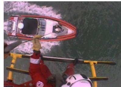
The actual course and speed will be confirmed by the helicopter pilot. The helicopter will maintain a head to wind aspect while matching the vessels speed and crabbing across the wind until directly overhead.
